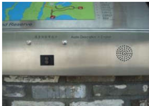
Figure 6-24: Speaker and buttons in talking signs
